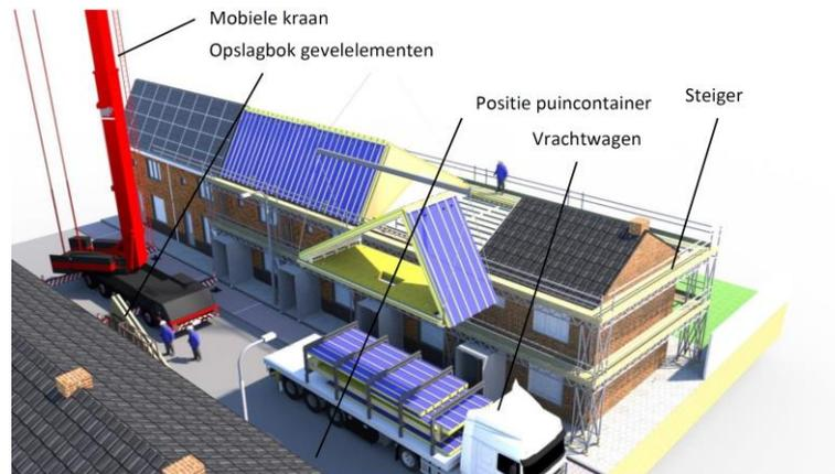
Figure 6: Fast retrofitting concept for roof of case 1.
